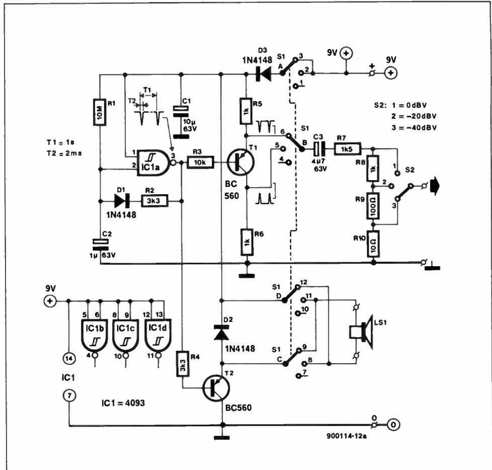
Fig. 2. Circuit diagram of the pulse transmitter.
