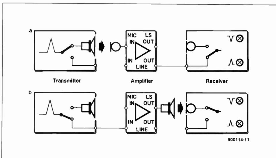
Fig. 1. Application examples of the phase-check system.
