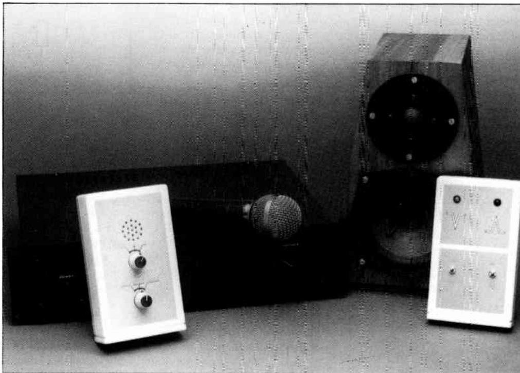
While setting up and connecting audio equipment it is important to have all the units — microphone, loudspeakers and everything in between — ‘in phase’, that is, interconnected with the right polarity. The low-cost instrument described here is particularly handy for checking out the phase of almost any audio system, whether installed in a living room, in a car, in a studio, or on a stage.
