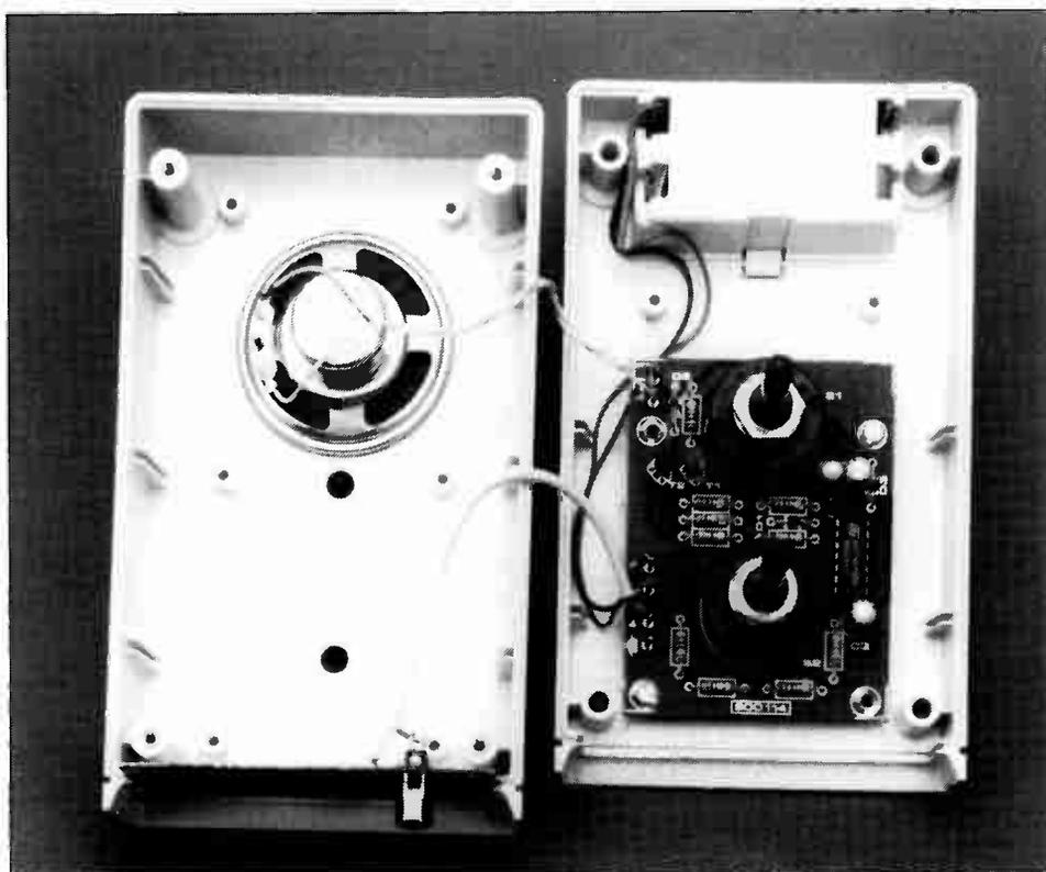
Fig. 5. A look inside the completed pulse transmitter.
