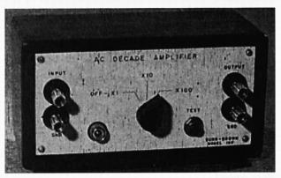
type-C flashlight cells are easily obtained. The instrument is decaded in gains of X10 and X100 and is accurate to plus or minus 0.2 db at 1 kc. Gain change on both ranges is less than 0.3 db throughout battery life. It has a frequency response of from 1 cps to 800 kc. The low B voltages needed for transistors make possible dc coupling which results in good low frequency response.
