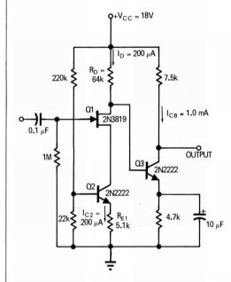
Unstable biasing method for FET Q1 direct coupled to bipolar transistor Q3. Constant-current source Q2 properly biases FET Q1 independently of its parameters  $I_{DSS}$  and  $V_{p}$ . Constant-current source Q2 determines FET drain current  $I_{p}$  and sets bias voltage at Q3 base. However, drift in Q2 collector current  $I_{c2}$  shifts base-bias voltage causing instability.
