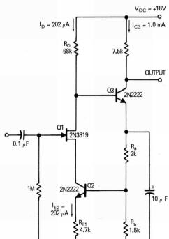
Stable Biasing Method incorporates dc-voltage feedback from Q3 emitter to base of constantcurrent stage Q2 to maintain stable bias voltage at Q3 base.
