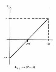
A single potentiometer controls the gain of an op amp over a bipolar range. The gain control is as linear as the pot.
