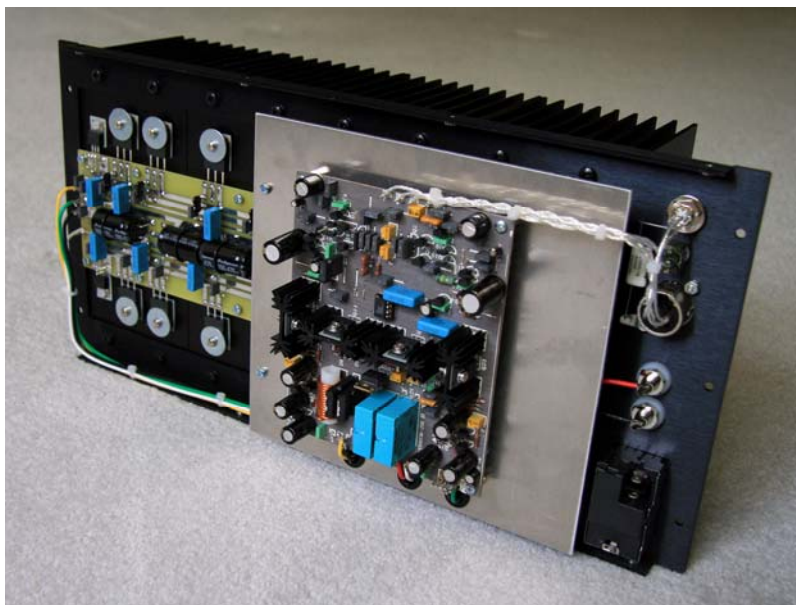
Millennium 200 Class AB Amplifier Rear Panel (In assembly)
